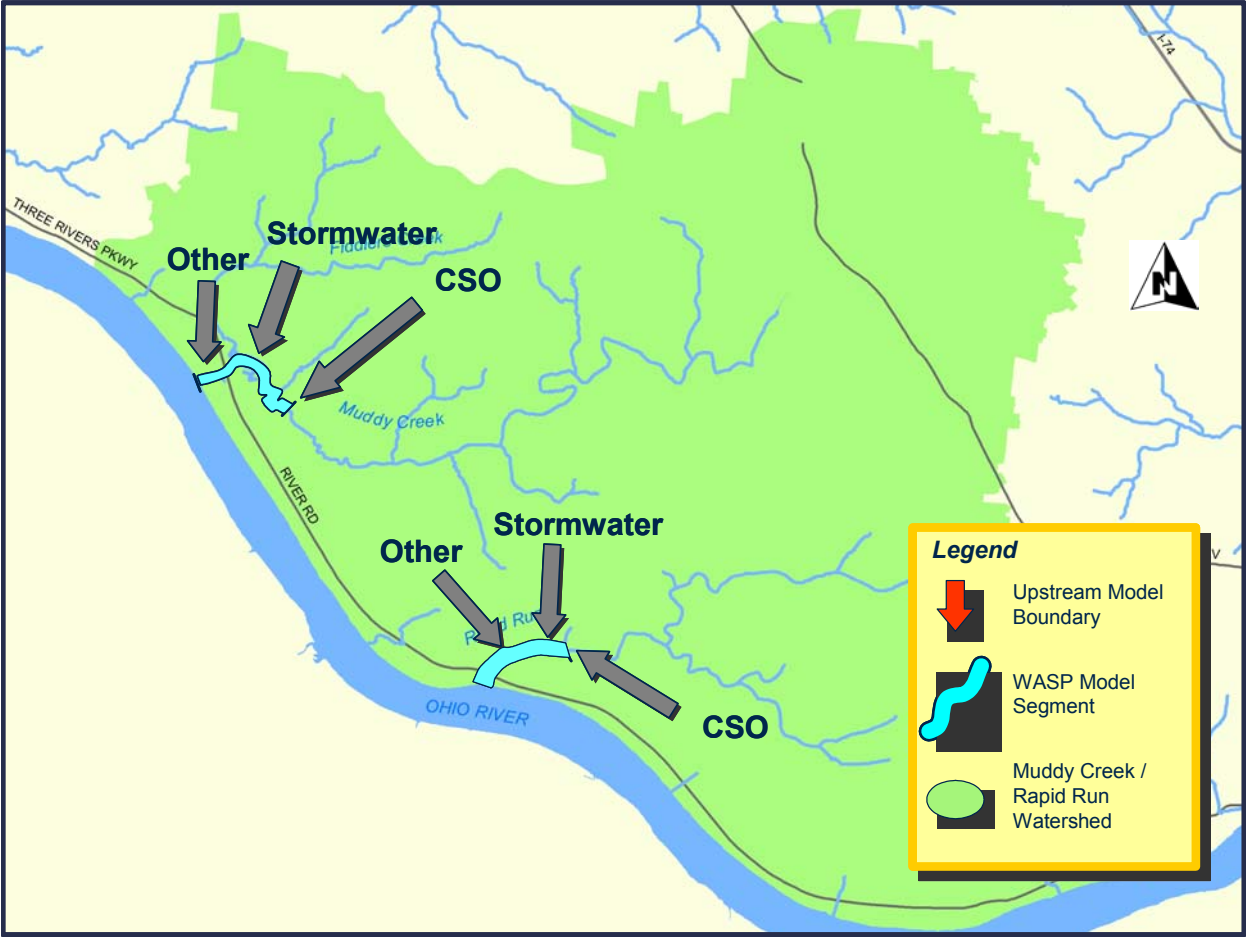
Exhibit 3: Figure 4 Conceptual Muddy Creek/Rapid Run WASP Model
